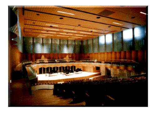
Shoebox shaped concert hall with 720 seats. Much glass area was introduced both to exterior and hall interior. Convexed glazing panels were installed on the upper side walls in the auditorium.
